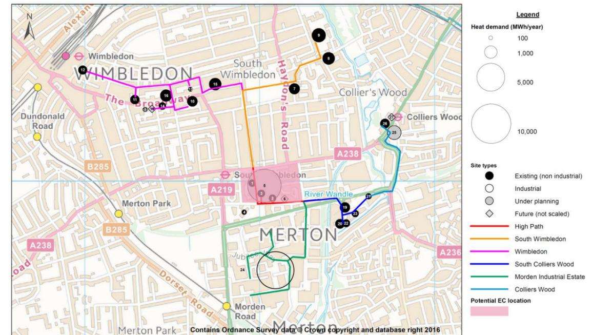
Figure 0-1: CWSW Network Options (building numbers provided in Table 7-1)
